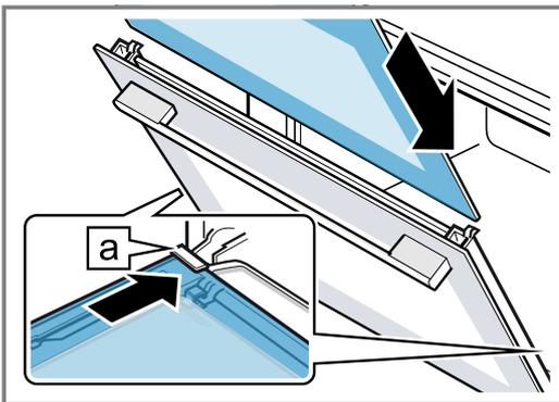
7. Push the inner pane upwards until it is in the left- and right-hand retainers [a].
