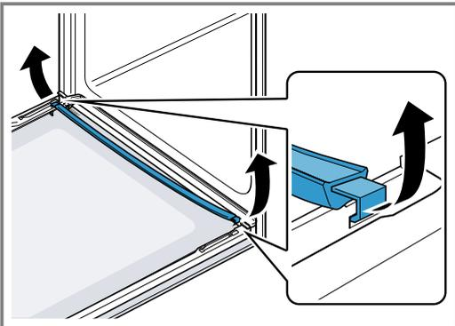
9. If necessary, you can remove the condensate trough for cleaning.
