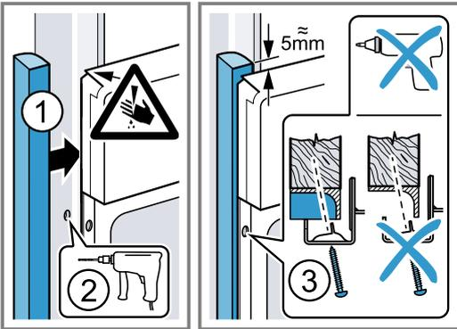
**Note:** The gap between the worktop and the appliance must not be closed by additional battens. Thermal insulation strips must not be fitted to the side panels of the surround unit.
