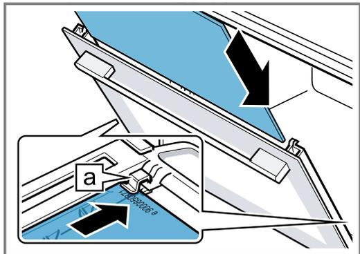
4. Push the intermediate pane upwards until it is in the left- and right-hand retainers [a].
