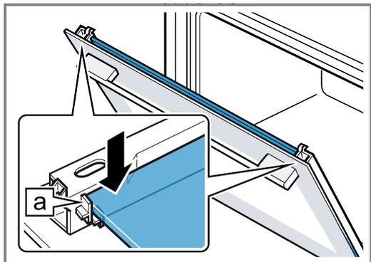
5. Open the appliance door and attach the door seal.
